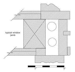
FIGURE 74. Section through exterior wall at window jamb. (T. Jones, NPS, 2005)
