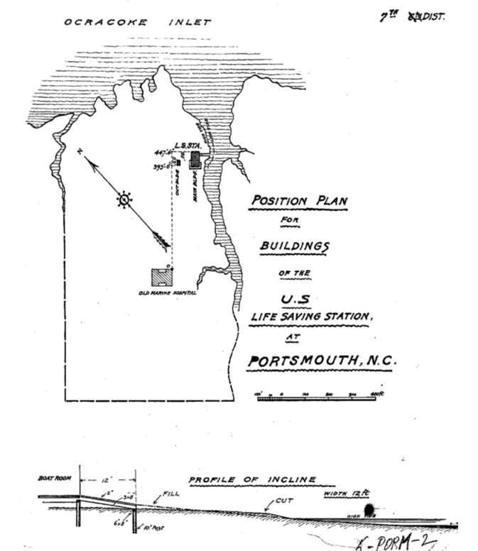
FIGURE 36. "Position Plan for Buildings of the U. S. Life-Saving Station at Portsmouth, N. C.," probably summer 1894. This plat is a revision of the plat of the proposed site that was drawn in July 1893 and shown in Figure 20. (National Archives and Records Administration, Philadelphia, PA, Record Group 26)
