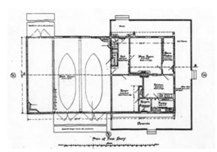
FIGURE 10. Tolman's plan for the station at the Columbian Exposition. (Taken from York, "Architecture of the United States Life-Saving Service")
